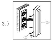
Step 3: Place the fixture on the back plate, and secure with two screws on the sides to hold the fixture in place. Caulk around back-plate where fixture meets the wall using outdoor silicone sealant. Leave a small gap at the bottom to allow moisture to escape.
