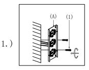
Step.1: Remove mounting bracket from fixture and install to electrical box.
