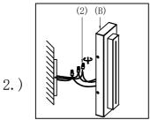
Step 2: Use wire nuts supplied to wire fixture to wires in outlet box. Copper wire is for Ground.
