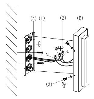
To prevent moisture from entering the outlet box and causing a short, seal around the top and side perimeter between the fixture and the wall surface with weather resistant caulking (see illustration a).
