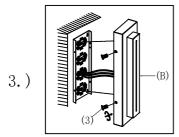
Step 3: Place the fixture on the back plate, and secure with two screws on the sides to hold the fixture in place. Caulk around back-plate where fixture meets the wall using outdoor silicone sealant. Leave a small gap at the bottom to allow moisture to escape.
